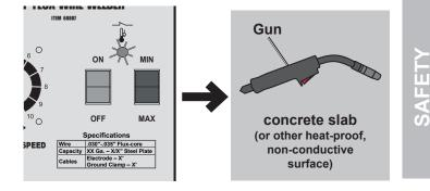
7. After welding the test weld on a piece of scrap for a few seconds, stop, and check your progress. Clean, then compare your weld's appearance with the diagrams and descriptions in the Welding Tips section starting on the next page. After making any necessary adjustments, continue to weld while carefully following the DUTY CYCLE guidelines as explained on page 14.
